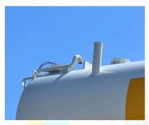
This elevated truck fill has an air gap in accordance with NAC 445A.
